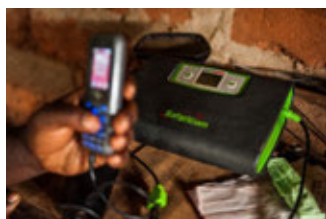
Figure 40: M-Kopa system charging a mobile phone
