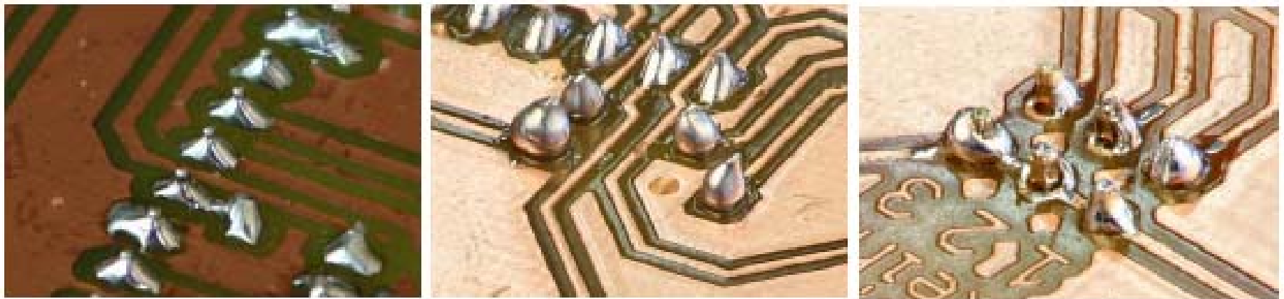
Figure 6-4: Good solder joints ( left ), cold joints ( center, in front ) and poor joints ( right ). 7
