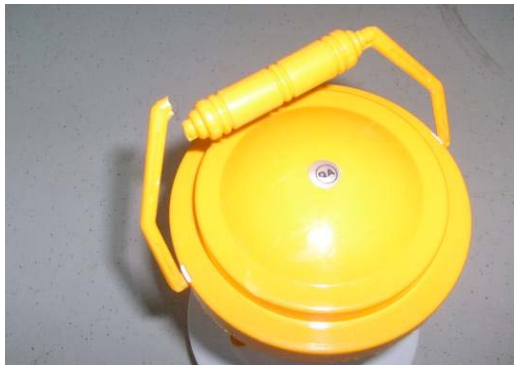
Figure 2-22: Broken handle following drop test.
