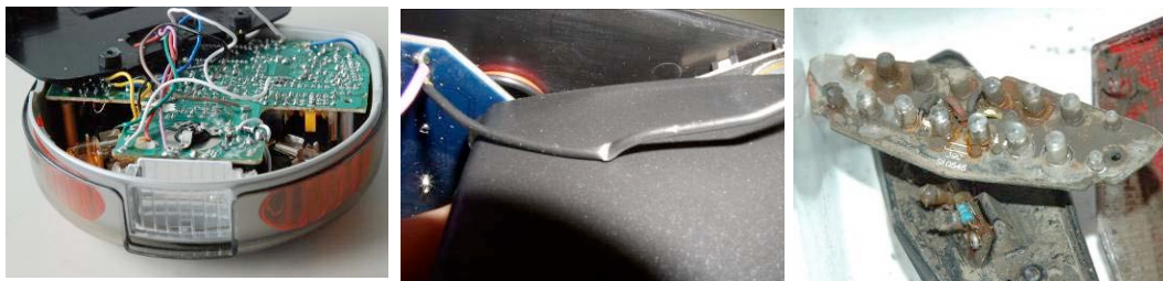
Figure 2-3: Cable spaghetti ( left ), wedged wire ( center ) and heavily corroded components ( right )
