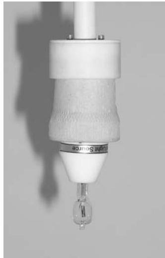
Figure 3-9: Standard calibration lamp correctly installed in the sphere's lamp socket.
